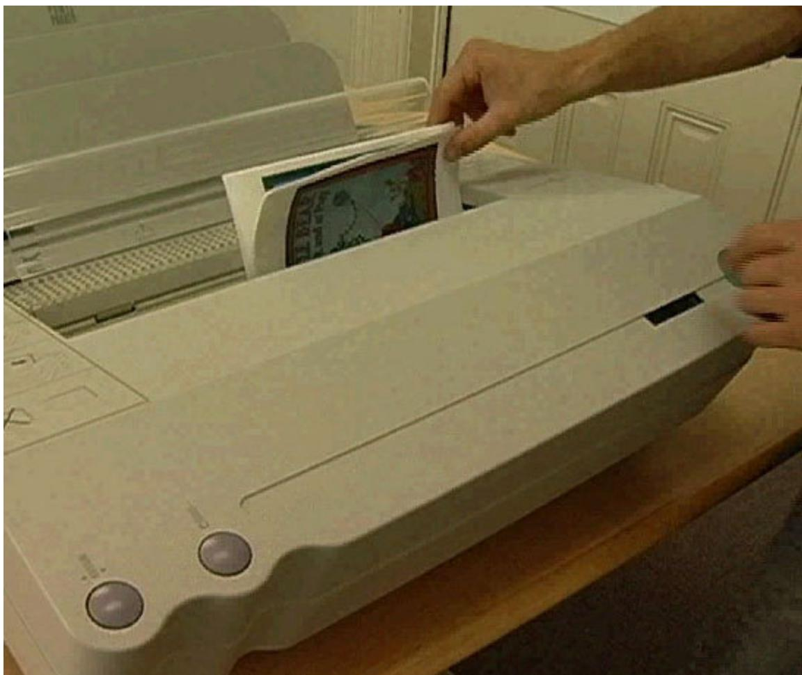
To score the cover, measure the width of the book on the orange measuring plate of the Powis Parker Scoring Machine. Place the cover into position one on the scorer, rotate the green ball to the left, exerting
